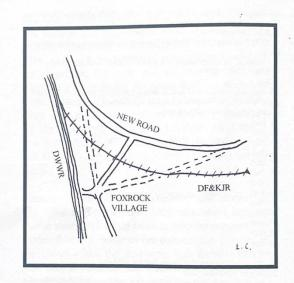
Proposal for junction at Foxrock Station, linking the new railway with the Dublin, Wicklow and Wexford Railway.
